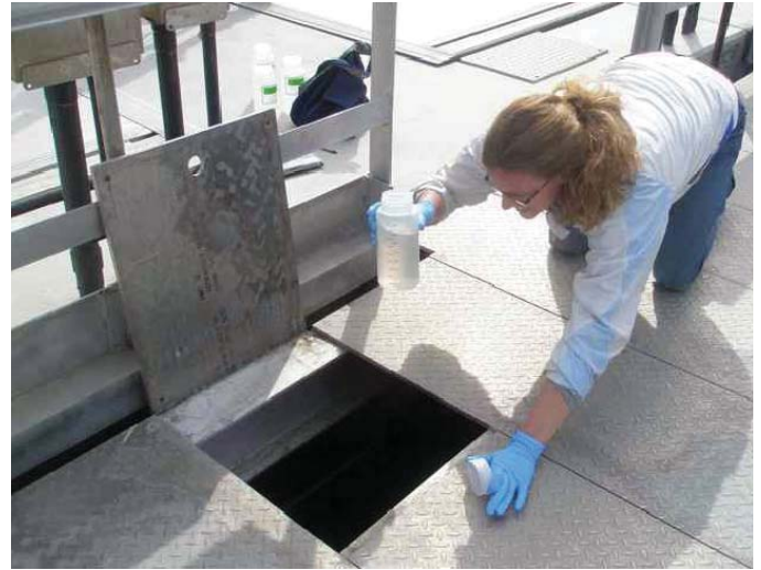
Stanford researcher Heather Bischel sampling the Watsonville, CA., wastewater treatment facility for analysis of perfluorochemicals.
